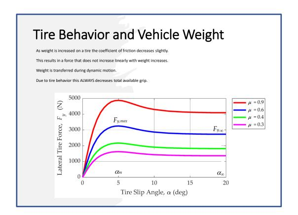
Adding a bit of weight to the tire increases its ability to grip the surface.....but, to a point. Past that point ....... grip decreases.
