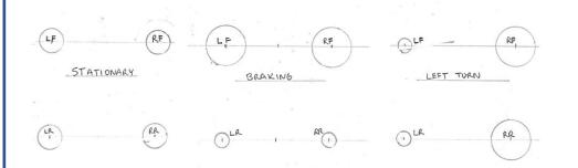
These diagrams show how weight is transferred between the 4 tires during Braking and a Left turn. The opposite occurs under Acceleration and a Right turn.
